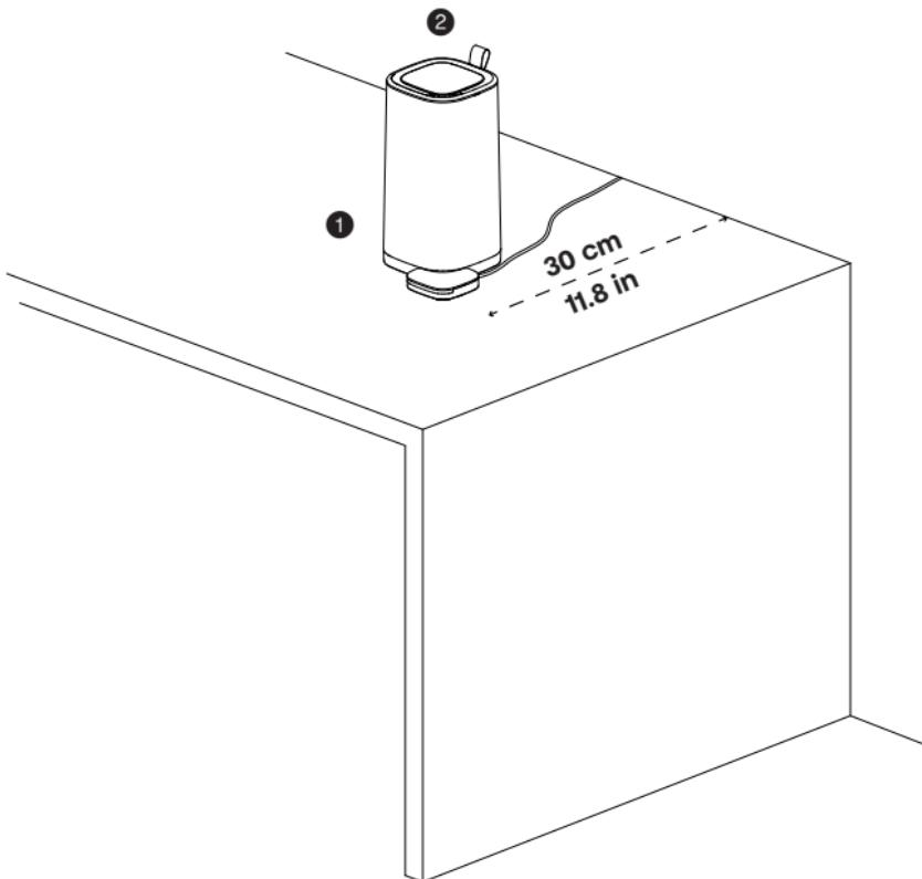
The Eteria system can be placed inside any room. Don't place it on the floor, near heat sources, and in environments with high humidity. We recommend placing it at least 30 cm/11.8 in from the wall. Don't obstruct the inlet ① and outlet ② area of the purifier. For accurate data, once positioned, don't move or turn off the air quality module.
