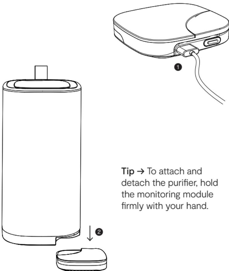
**Tip →** To attach and detach the purifier, hold the monitoring module firmly with your hand.
