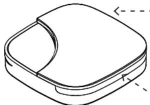
**Sensors** → Temperature (T), humidity (HR), volatile organic compounds (TVOC), carbon dioxide (CO<sub>2</sub>).
